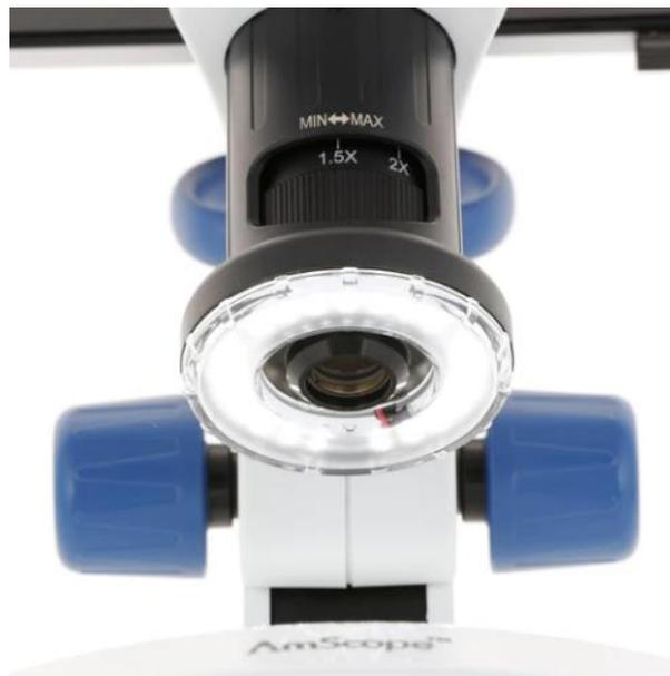
This microscope is equipped with an LED ring light and an under-stage LED light array to provide illumination. The ring light is fixed in place around the objective lens. The under-stage light array is fixed in place underneath the stage plate of the microscope, and it can be useable when the glass stage plate is in place under the objective rather than the plastic opaque stage plate.
