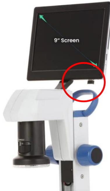
The microscope has one USB port on the right underhand side of the monitor. This is used to connect the included mouse. The microscope also has one micro SD card slot on the right side of the monitor, labelled TF-Card.
