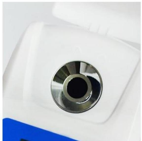
**04** Clean and dry the sample tank for the next measurement
